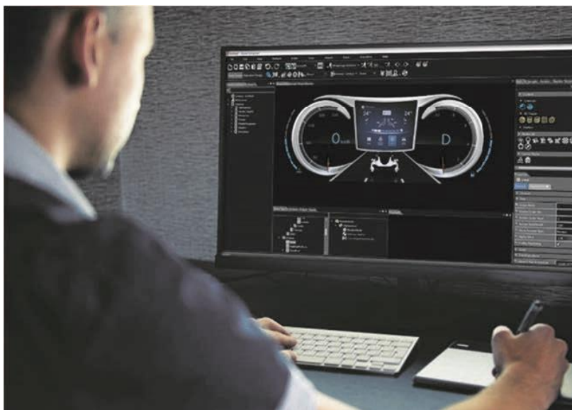
Fig1: CGI Studio is a Software platform for development of 2D/3D automotive HMIs
